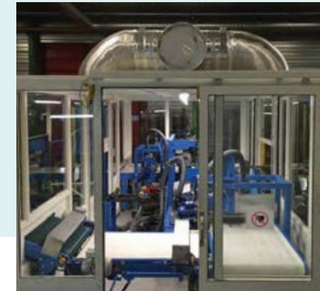
Drums are cleaned with pressurized air at one of Greif's plants in France. The process uses no cleaners, reducing its impact on the environment.
